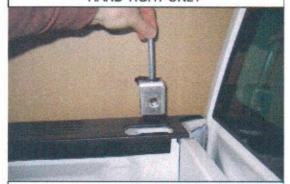
HAND THREAD 3/8" X 4" BOLT INTO STAKE POCKET BRACKET & LOWER INTO STAKE HOLE AS SHOWN.
