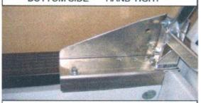
USE INDICATED BOLT THROUGH THE PROPER FRONT HOLE INTO STAKE POCKET BRACKET. TIGHTEN J-HOOK BOLT FIRST, THEN FRONT BOLT - FINISH TIGHTENING 5/8" BOLT THROUGH INSIDE OF BED TO STAKEPOCKET BRACKET.
