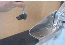
USE 3/8" X 2" BOLT, LOCK WASHER & 5/16" FLATWASHER THROUGH THE REAR SLOTTED HOLE WITH THE J-CLAMP ON THE BOTTOM SIDE \*\* HAND TIGHT \*\*
